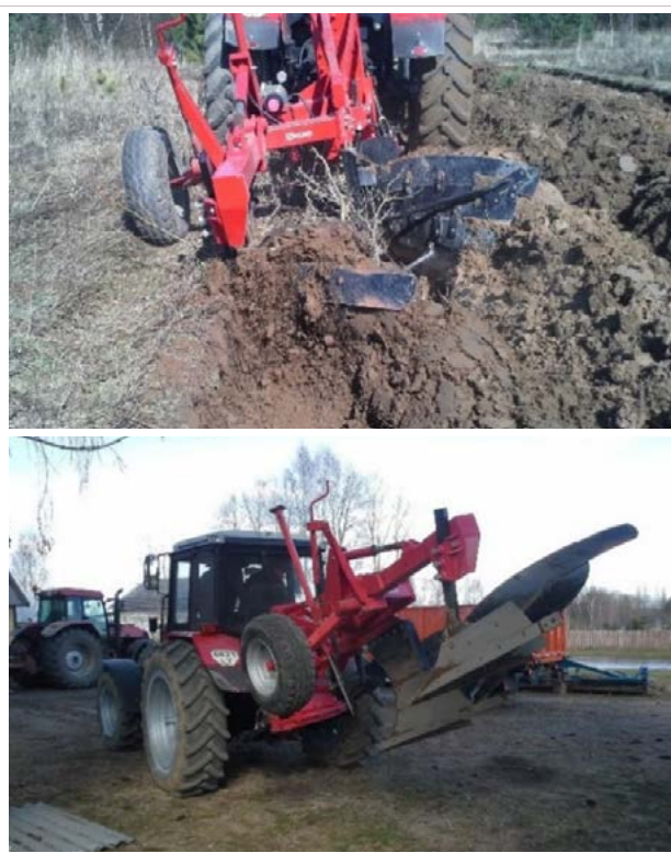
Figure 2. Example of deep inversion ploughing with Bovlund-80 deep ploughs (Photos: Gediminas Survila)
