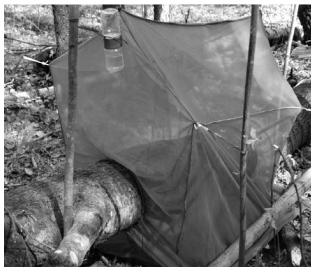
Figure 1. Emergence trap set on fallen tree trunk
